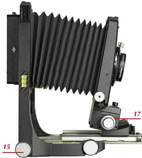
Above: The Linhof Techno with Scheimpflug adjustment (tilt) at the lens standard with micro drive (17). When using lenses with reduced image circles we additionally recommend to shift the rear standard up with the micro drive (15).
